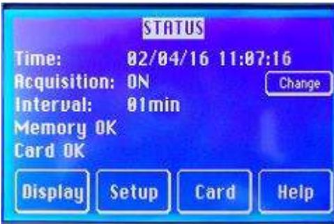
The **Display** button allows viewing of current values.
