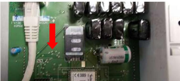
To insert the modem SIM card, unscrew the 4 screws and lift the front panel. Open the SIM card cover by sliding it towards the arrow direction.
