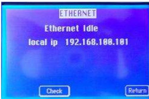
If idle it shows the instrument's IP address.
