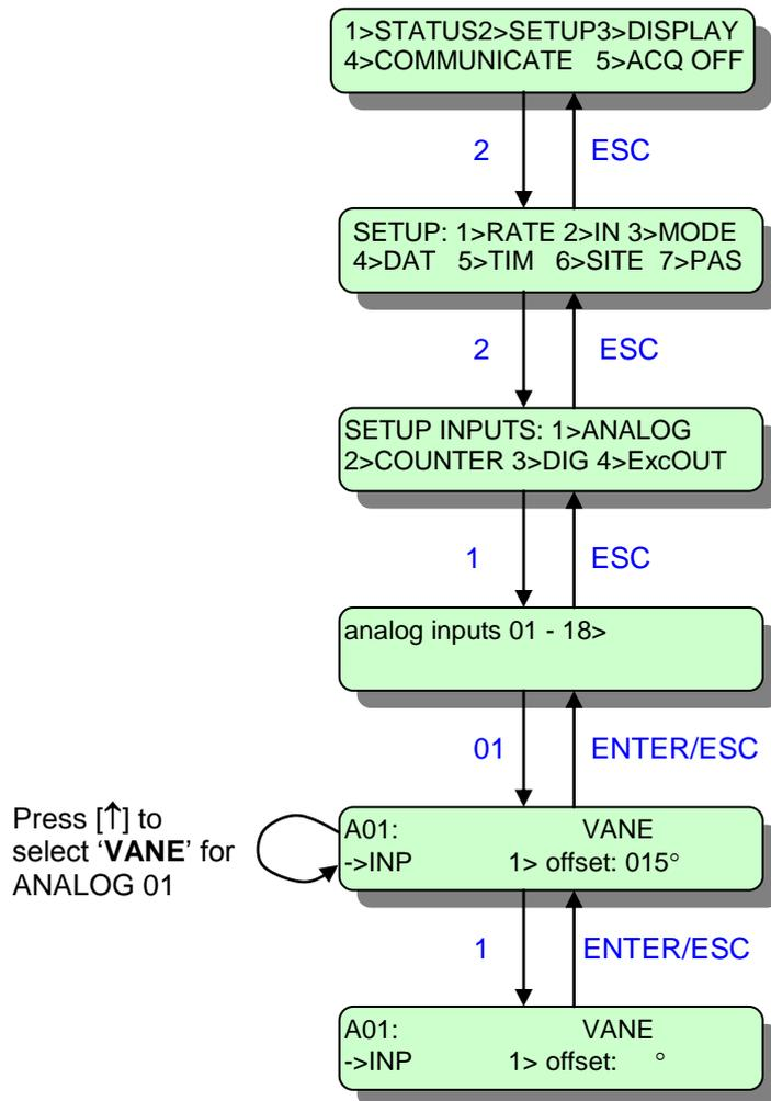
Enter the vane offset for direction measurement in degrees (0~359). For instance, if the vane “zero” mark is placed 30 east then you enter 30 as offset; if it is placed 30 West you enter 330 (=360-30) as offset.
