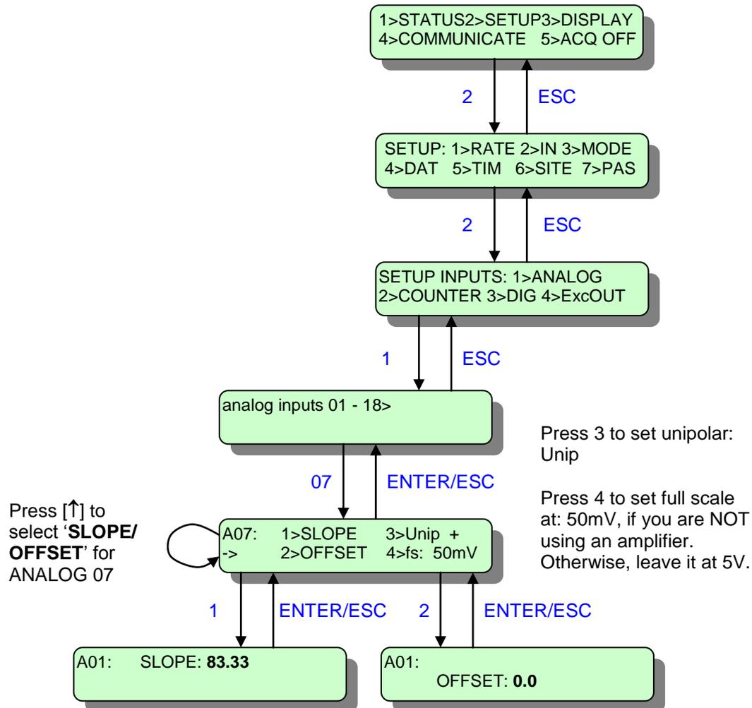
Set Slope=83.33, if you are NOT using an amplifier. Otherwise, set Slope=0.7184 .
