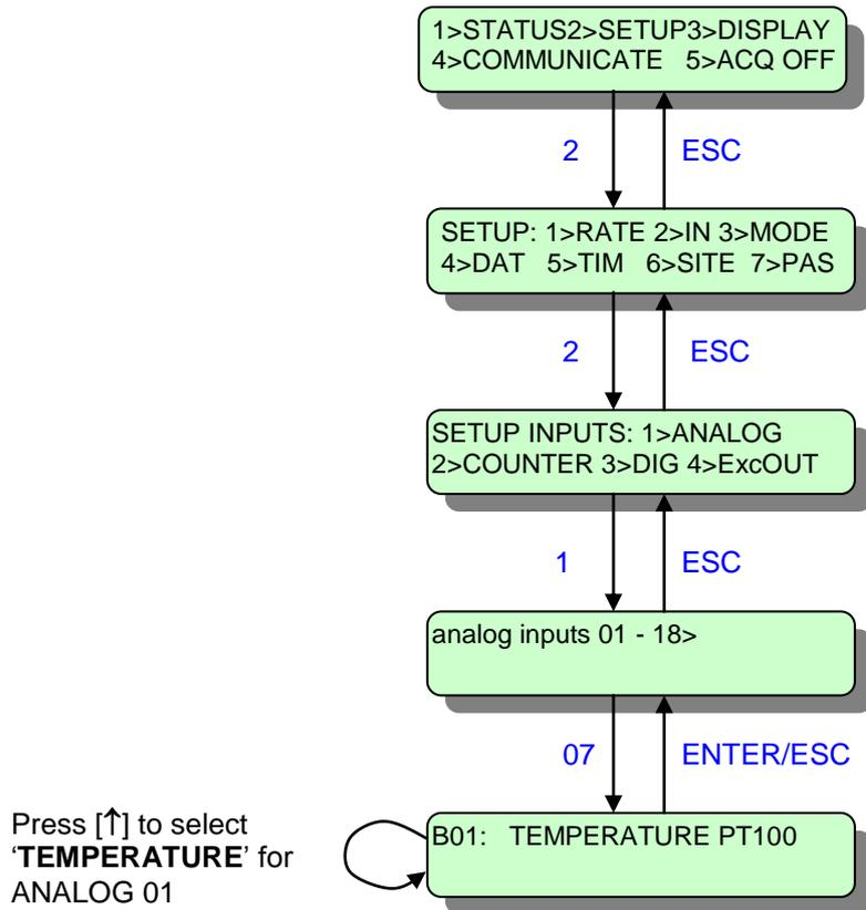
Press [-] to select bridge **(B01)** configuration for ANALOG 01
