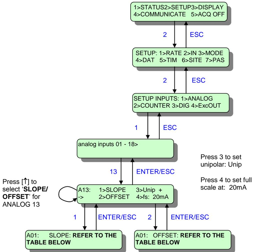
For calibrated sensors enter the correct SLOPE and OFFSET values.
