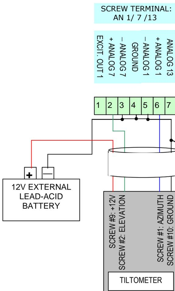
In order to have the Azimuth display 0 degrees when the mast tilts North, fasten the Tiltometer such, that in vertical position the box label 'looks' South.
