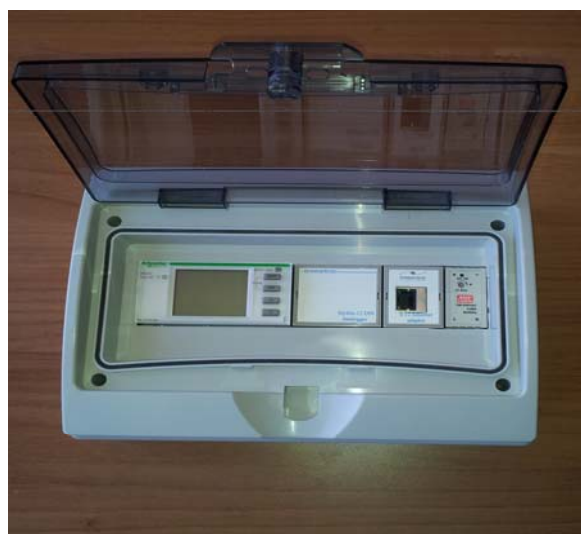
DIN rail system with MODBUS multimeter, data logger Ethernet adaptor and power supply.
